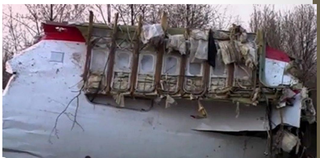
Cokpit and front part of fuselage are not inverted
