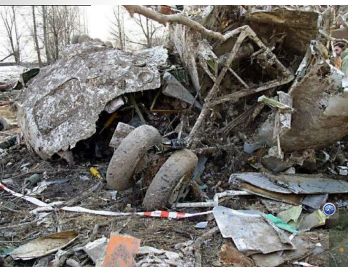
Cokpit and front part of fuselage are not inverted
