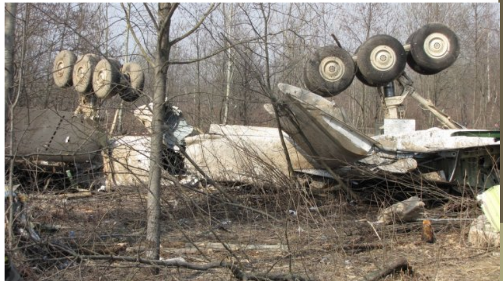
Rear parts of the fuselage in inverted position
